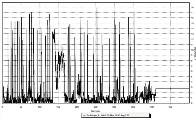
In the example above, the average current was 2.62 amps, which calculates to 435mAh per 10 minutes (typical flight length). It's recommended that only 60% of the available capacity be used to ensure plenty of reserve battery capacity. In this example, using two 4000mAh batteries (8000mAh total capacity)  $\times$  60% = 4800mAh (available usable capacity) divided by the capacity used per 10-minute flight. 435mAh would allow up to 11 flights of 10 minutes each.
