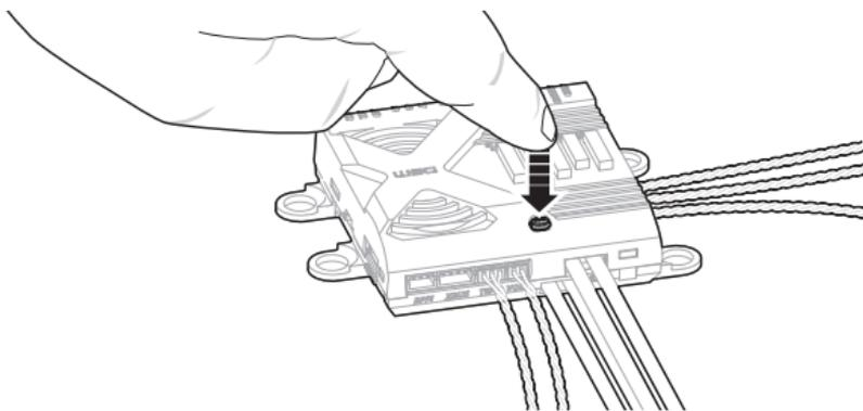
**NOTICE:** If using a bind plug, remove the bind plug after binding to prevent the system from entering bind mode the next time the power is turned on.
