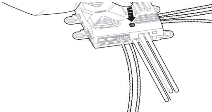
**NOTICE:** If using a bind plug, remove after binding to prevent the system from entering bind mode the next time the power is turned on.
