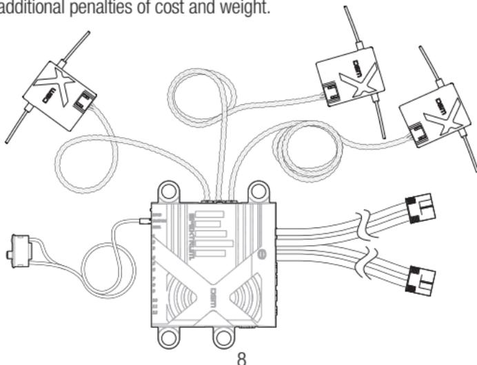
1. Using foam or thick double-sided foam tape and tie wraps, secure the main PowerSafe unit in the position where you would normally mount the receiver.
