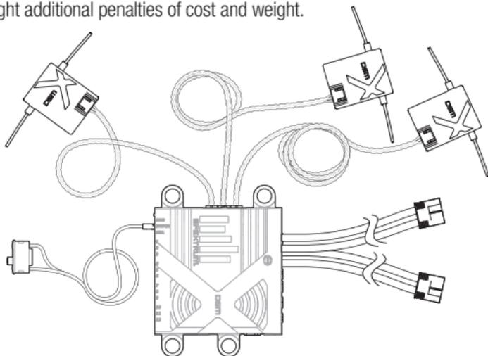
1. Using foam or thick double-sided foam tape and tie wraps, secure the main PowerSafe unit in the position where you would normally mount the receiver.
