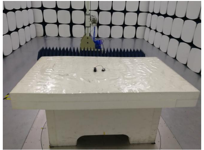
Radiated Emissions Test Setup Above 1GHz
