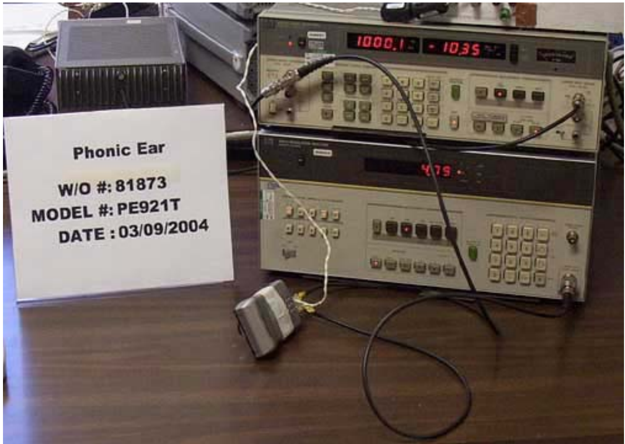
PHOTOGRAPH SHOWING AUDIO MODULATION TEST SETUP
