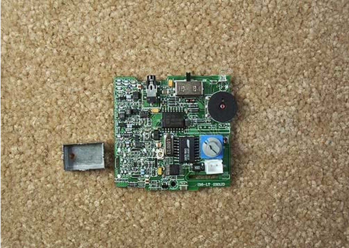
Main PCB Top with no Can of Small PCBs
