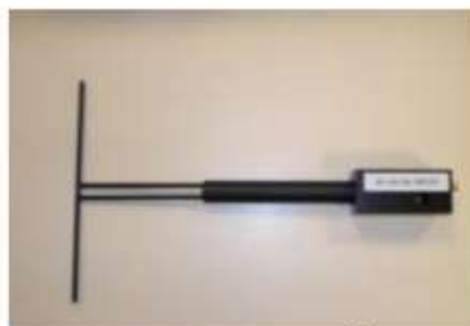
Figure 1 – Satimo COMOSAR Validation Dipole
