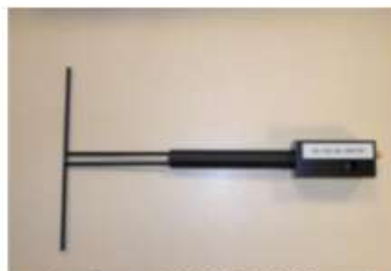
Figure 1 – Satimo COMOSAR Validation Dipole
