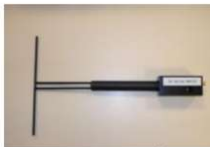
Figure 1 – Satimo COMOSAR Validation Dipole
