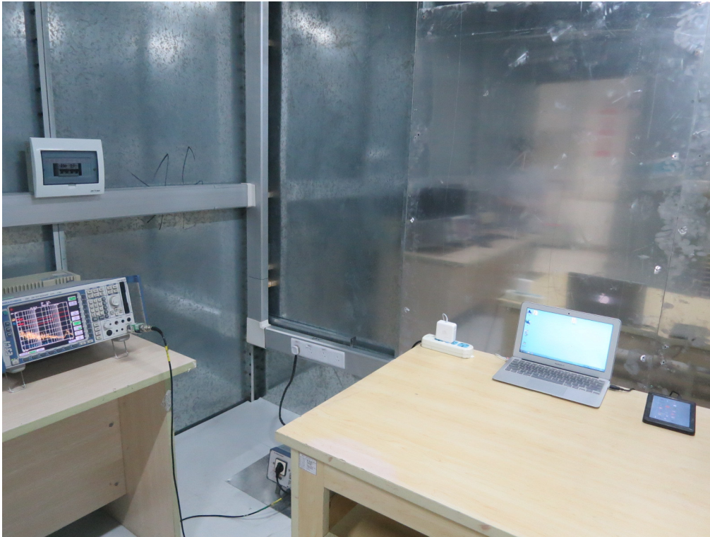
FCC RADIATED EMISSION TEST SETUP
