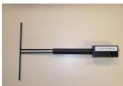
Figure 1 – Satimo COMOSAR Validation Dipole
