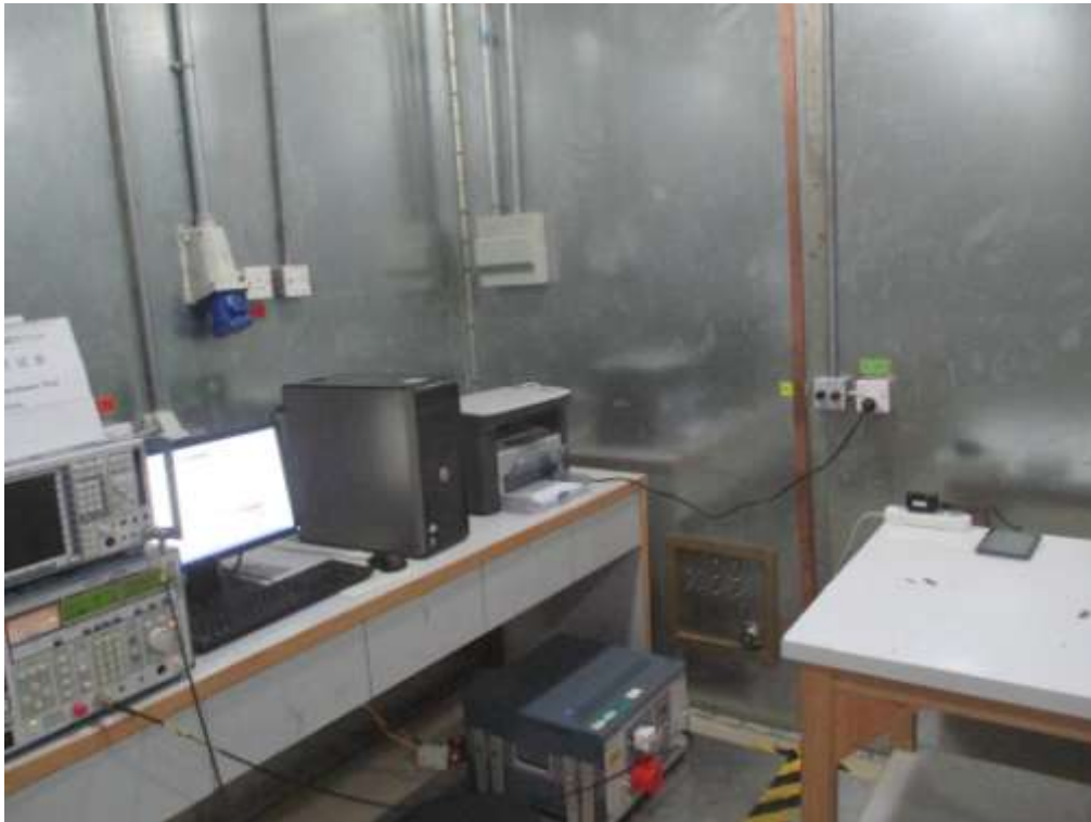
FCC RADIATED EMISSION TEST SETUP
