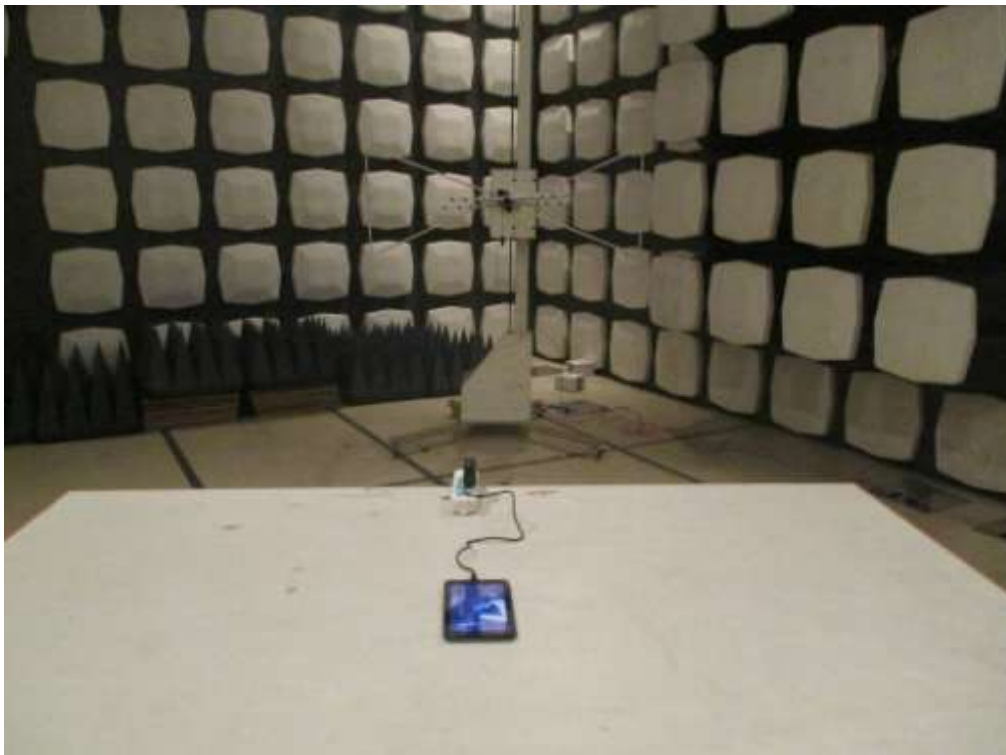
FCC RADIATED EMISSION TEST SETUP
