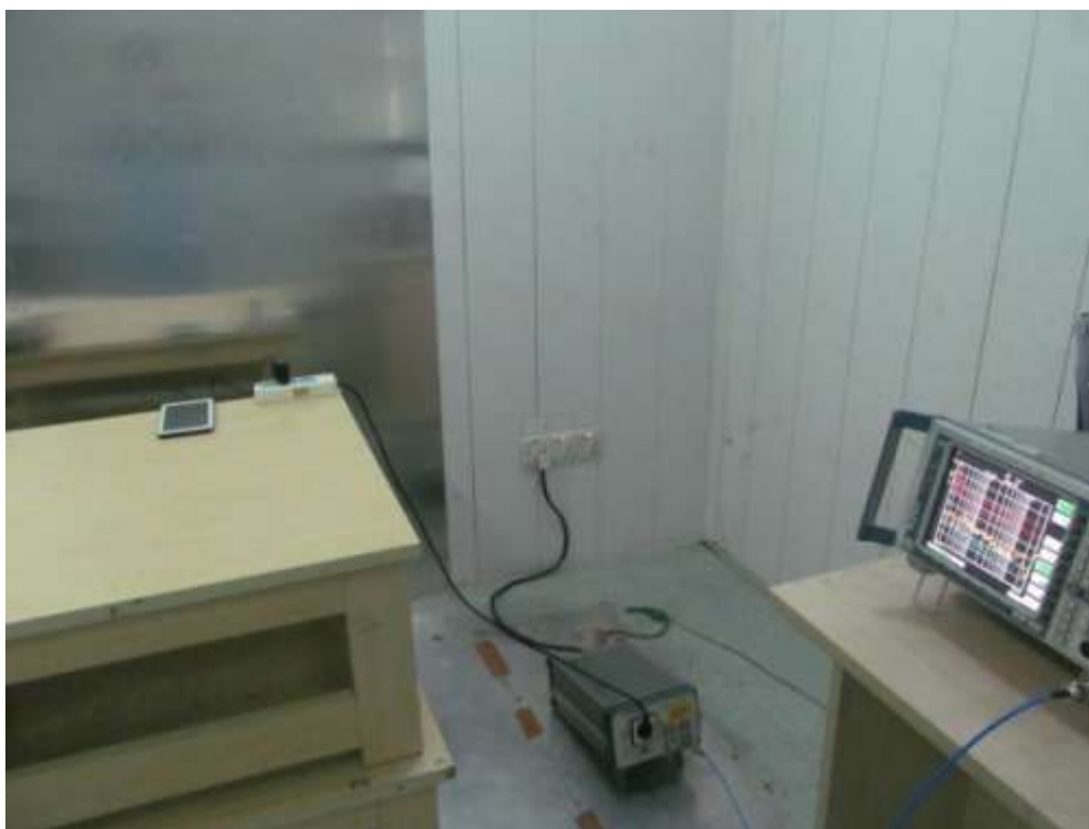
FCC LINE CONDUCTED EMISSION TEST SETUP
