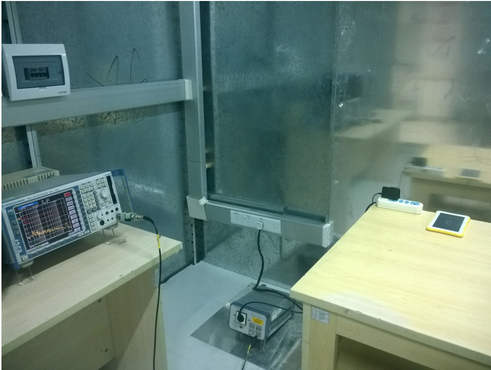
FCC RADIATED EMISSION TEST SETUP
