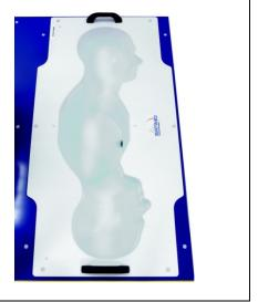
The bottom plate contains three pair of bolts for locking the device holder. The device holder positions are adjusted to the standard measurement positions in the three sections. A white cover is provided to tap the phantom during off-periods to prevent water evaporation and changes in the liquid parameters. On the phantom top, three reference markers are provided to identify the phantom position with respect to the robot.
