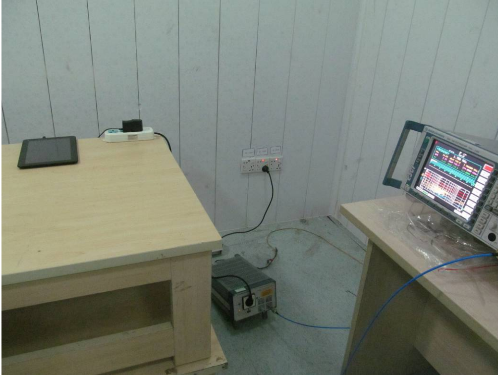
FCC LINE CONDUCTED EMISSION TEST SETUP
