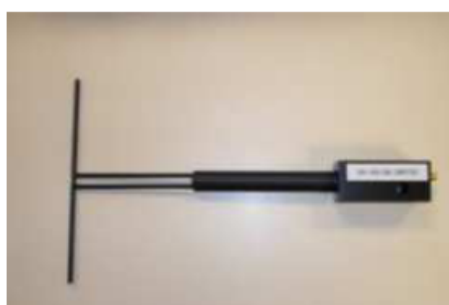
Figure 1 – Satimo COMOSAR Validation Dipole
