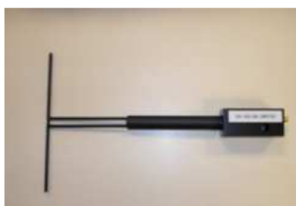
Figure 1 – Satimo COMOSAR Validation Dipole
