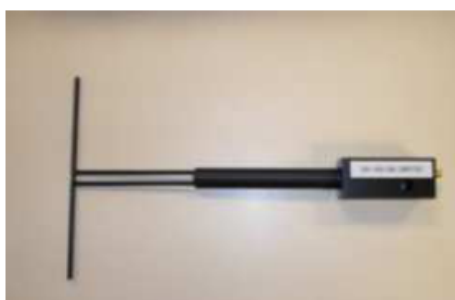
Figure 1 – Satimo COMOSAR Validation Dipole
