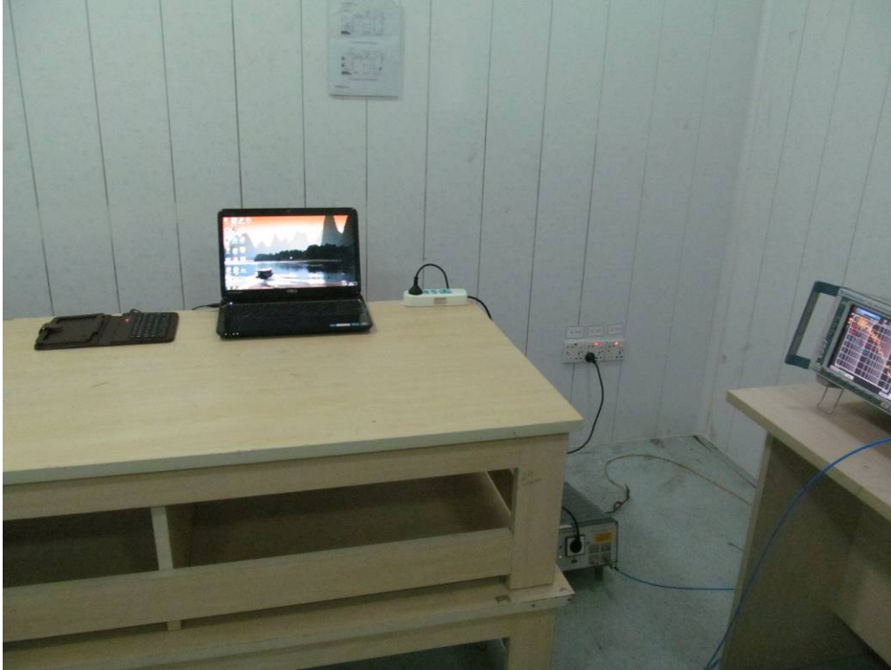
FCC LINE CONDUCTED EMISSION TEST SETUP
