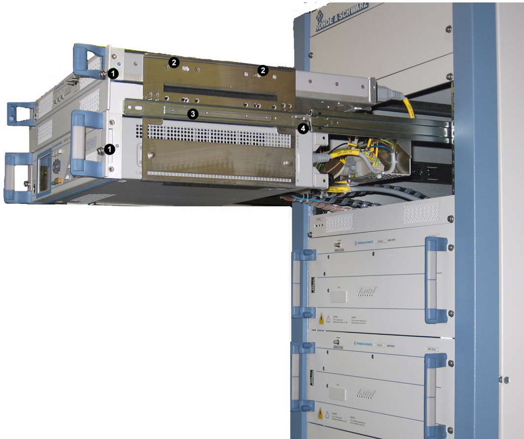
Fig. 14 Removing the exciter from the transmitter rack
