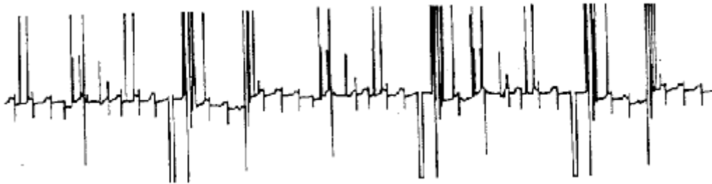
Fig. 99. Example 4 - Electrode Contact Noise
