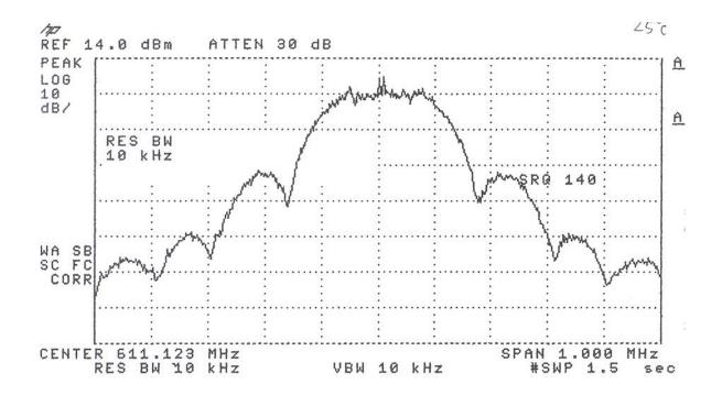
PLOT 2 (25 degrees C temperatore with supply voltage set to 115% of nominal)
