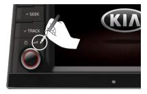
Press the reset hole using a clip or pin.
