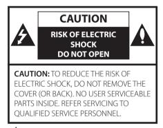
The lightning flash with the arrowhead symbol within an equilateral triangle is intended to alert the user about the presence of uninsulated dangerous voltage within the product's enclosure that may be of sufficient magnitude to constitute a risk of electric shock.
