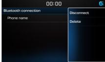
Press and hold the phone name to disconnect/ delete the device
