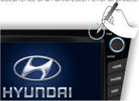
Press and hold the RESET key for about 1 second. (The use of a clip or pin is recommended when resetting the system.)
