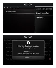
From the Bluetooth<sup>®</sup> device, search for the car name and pair the device. When searching from the Bluetooth<sup>®</sup> device, the car name is KIA MOTORS and the default passkey is '0000'.
