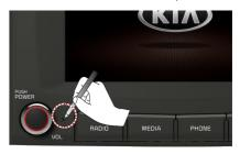
Press and hold the RESET key for about 1 second. (The use of a clip or pin is recommended when resetting the system.)
