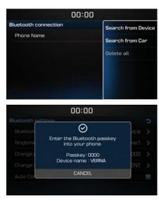
From the Bluetooth<sup>®</sup> device, search for the car name and pair the device. When searching from the Bluetooth<sup>®</sup> device, the car name is VERNA and the default passkey is '0000'.
