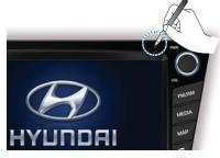
Press and hold the RESET key for about 1 second. (The use of a clip or pin is recommended when resetting the system.)
