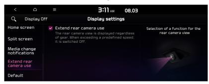
When you shift to "P" (Park) or drive at a predetermined spped or faster, the rear view display disappears to display the previous screen.
