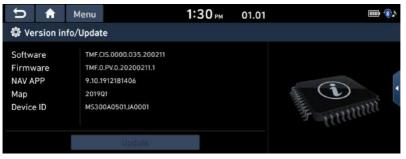
2. After inserting the USB with the update file, press [Update]. Once updating is complete, the system will automatically restart.
