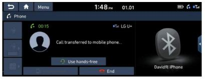
If you want to switch the call to the car hands-free while talking on the mobile phone, press [Use hands-free] on the screen or press and hold [ ] on the steering wheel remote control. The call is switched to the car hands-free.
