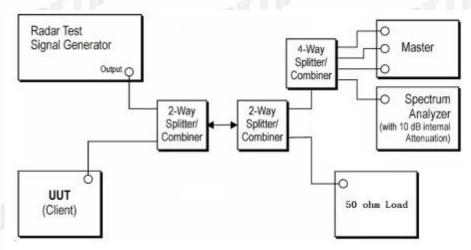
Note: 1. Use the software "Web" to set the frequency channel.
