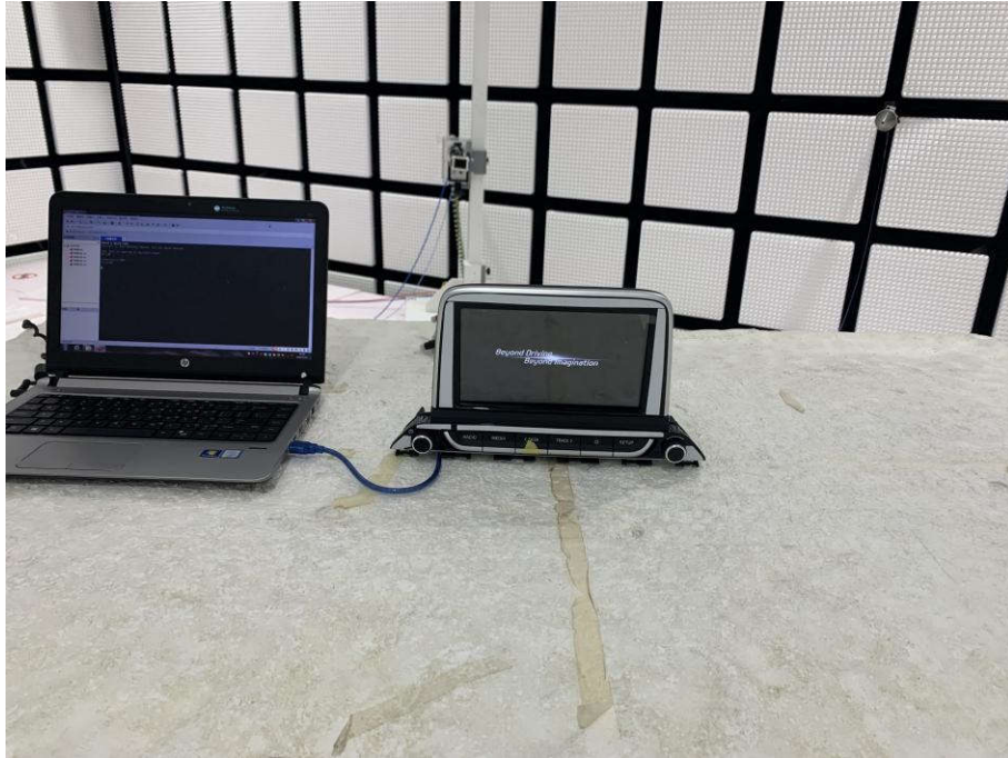
Radiated spurious emission Test Setup-3(Above 18GHz)
