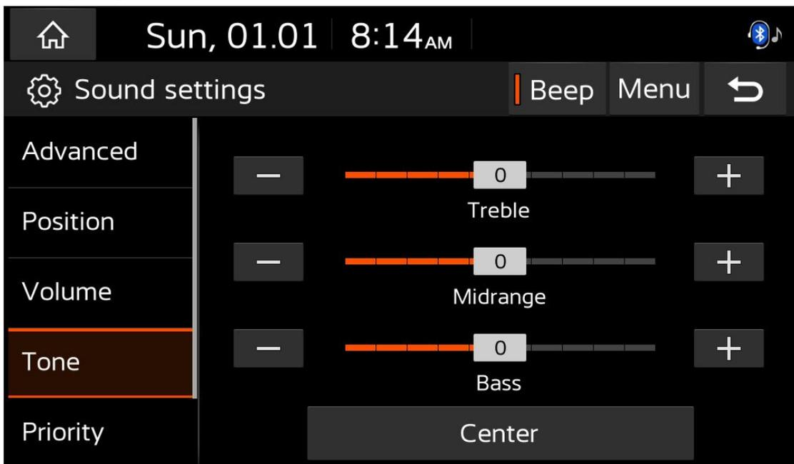
This menu allows you to set the [Treble]/[Midrange]/[Bass]. It can be adjusted by clicking the plus / key button.
