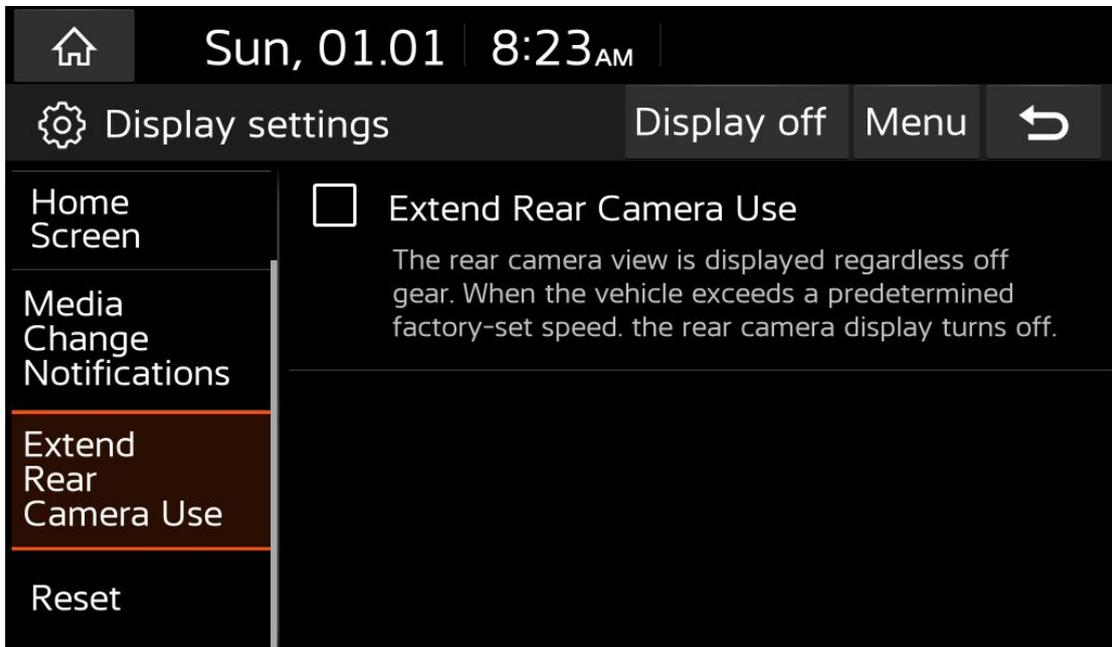
When the vehicle speed exceeds the preset factory set speed, the rear camera is off.
