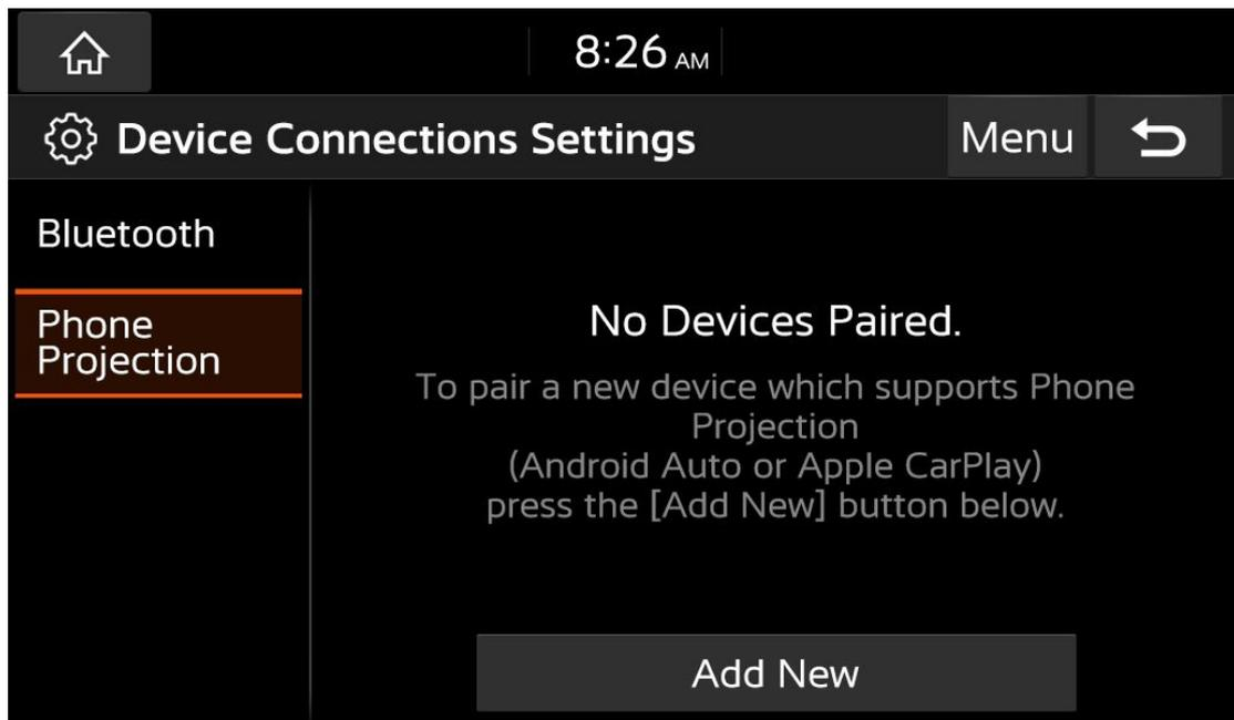
Click [add new] to search for available wireless carplay devices. Press the cancel button to stop the search. You can pair up to 8 devices. Click the Connect button to connect to the paired device, and click the Delete button to delete the paired device.
