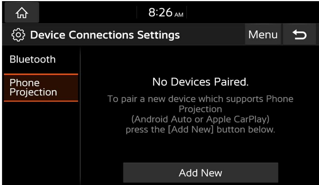
2. Click [add new] to search for available wireless carplay devices. Press the cancel button to stop the search. You can pair up to 8 devices. Click the Connect button to connect to the paired device, and click the Delete button to delete the paired device.
