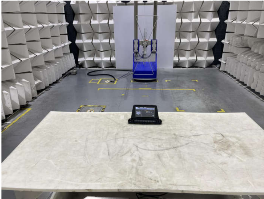
Radiated spurious emission Test Setup-1(Below 1GHz)
