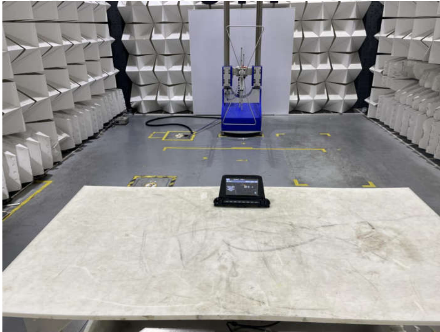
Radiated spurious emission Test Setup-1(Below 1GHz)
