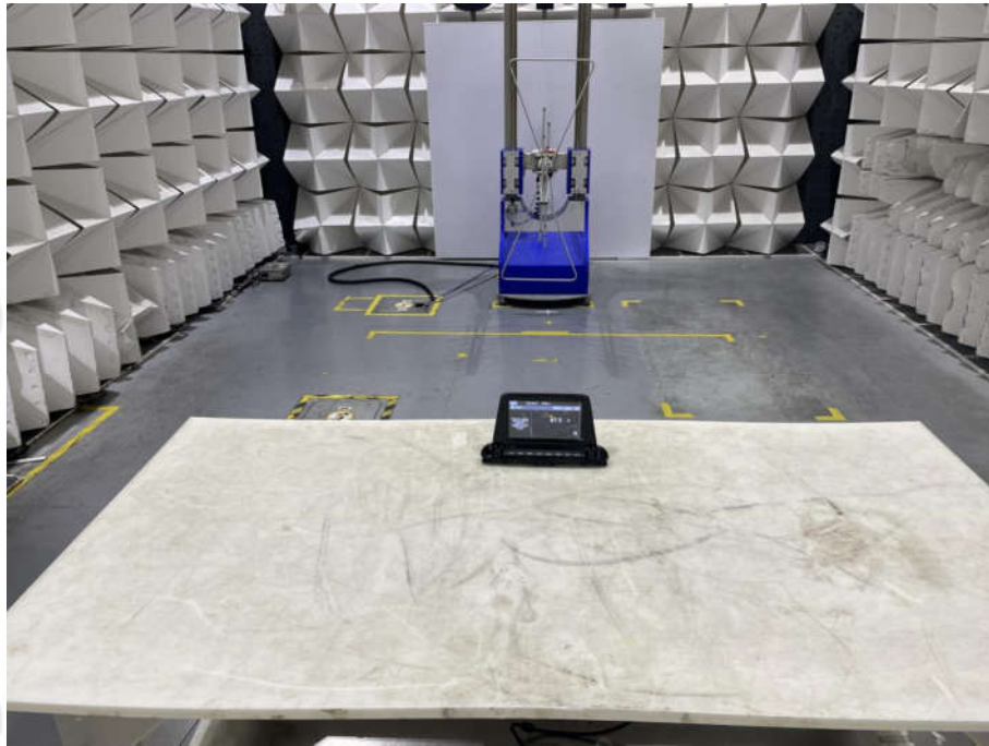
Radiated spurious emission Test Setup-1(Below 1GHz)
