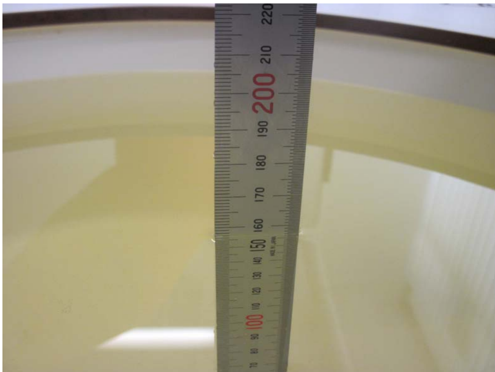
Picture B2 Liquid depth in the Flat Phantom (2450MHz)
