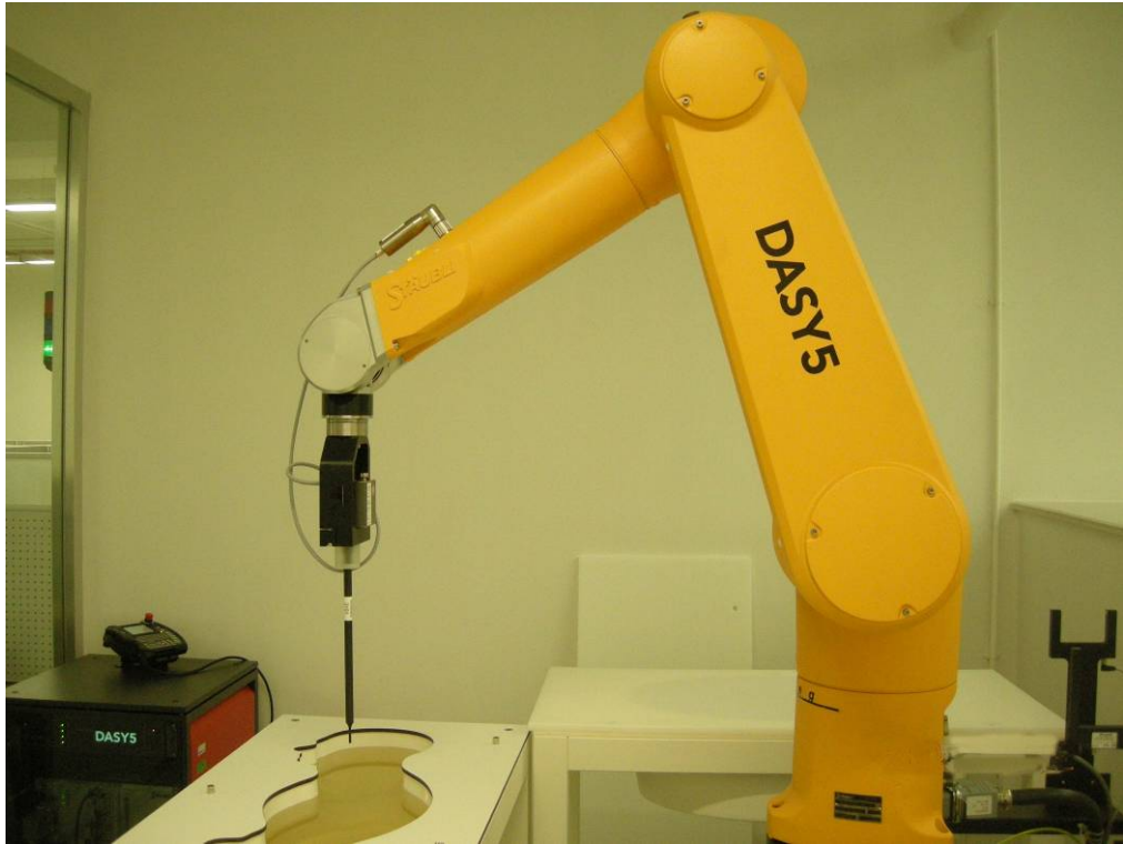
Picture B1: Specific Absorption Rate Test Layout
