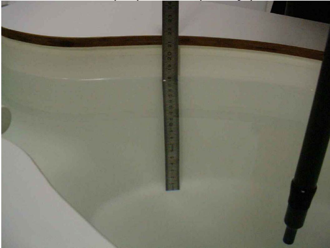
Photo 10: Liquid depth 2450 MHz body simulating liquid
