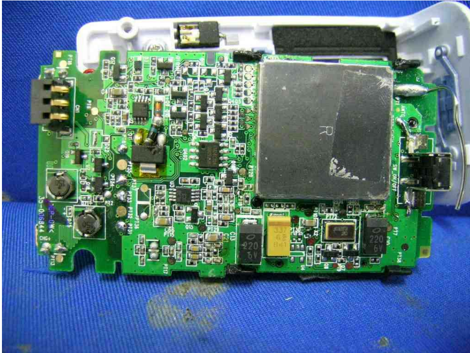
Parent Unit Main PCB comp side
