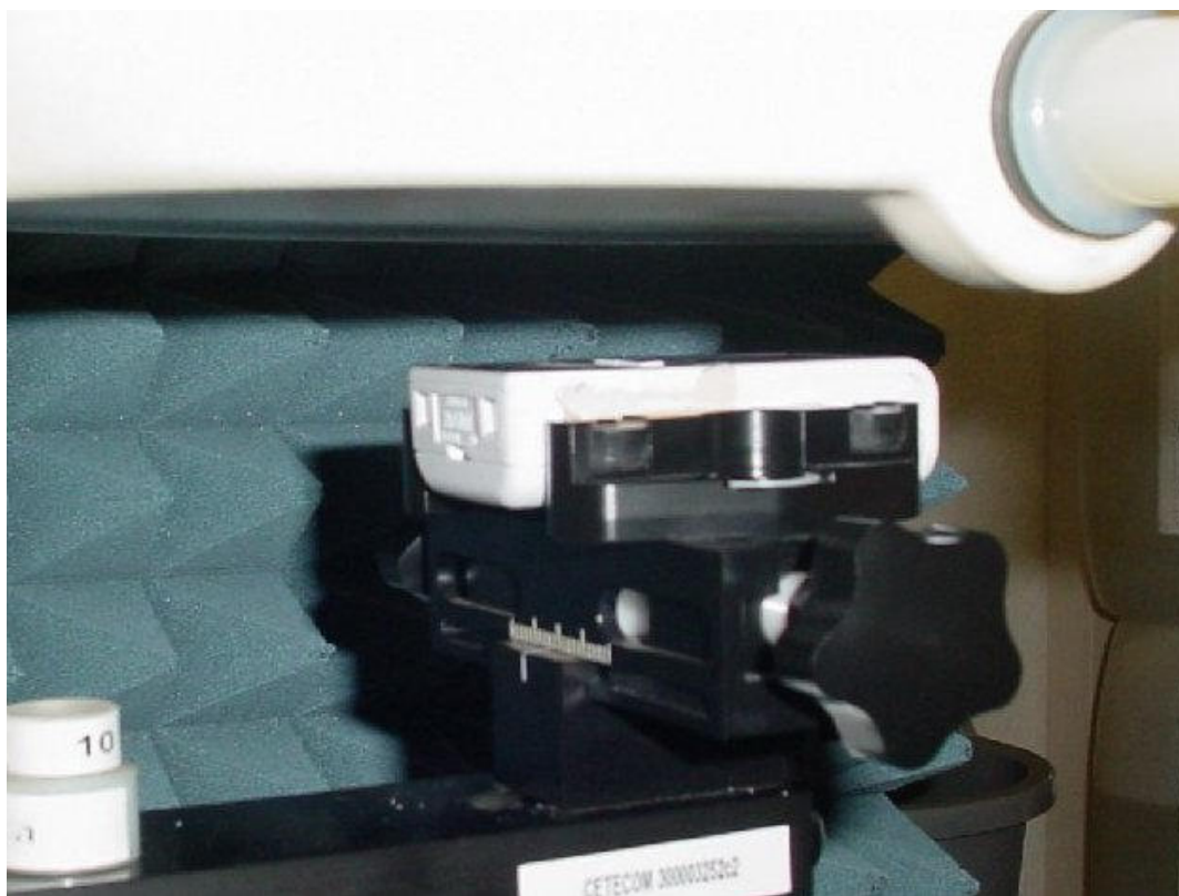
Photo 10: Test position front side with 25 mm distance
