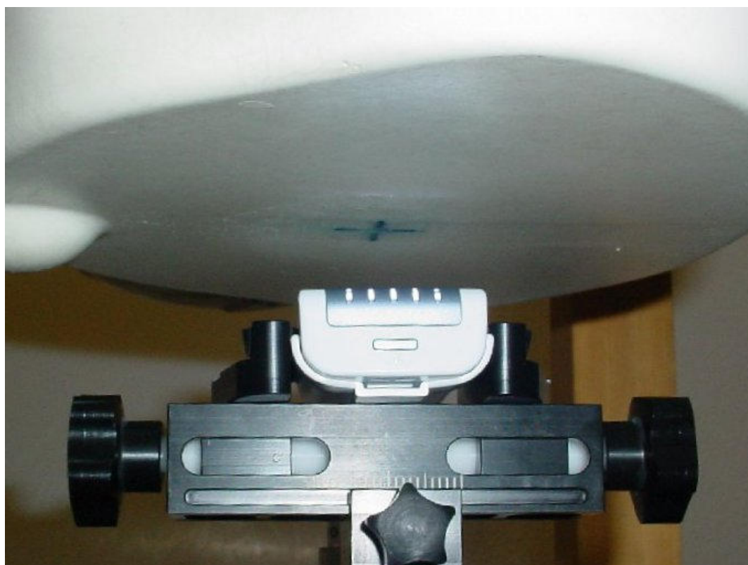
Photo 10: Test position front side with 25 mm distance
