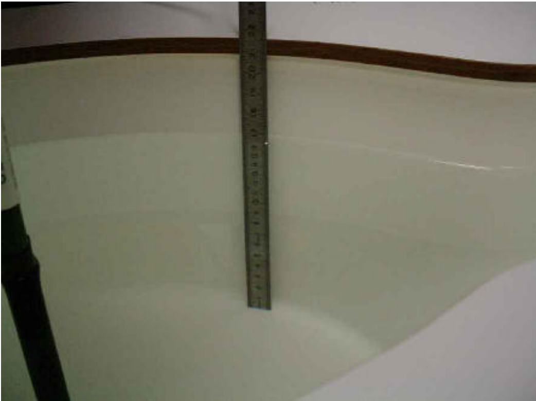
Photo 16: Liquid depth 1900 MHz body simulating liquid
