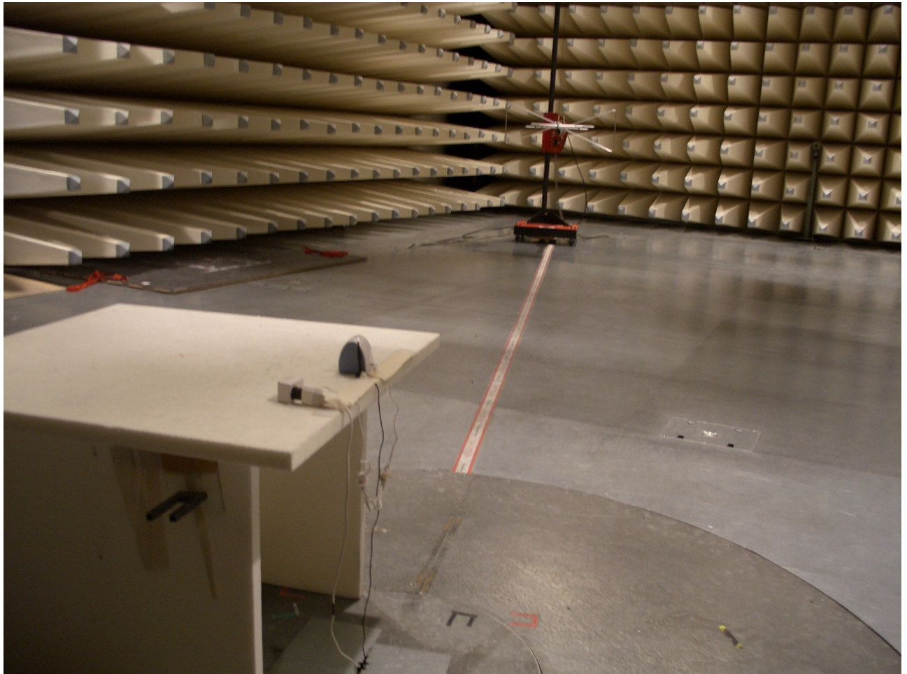
Photo 2: Radiated Emission and Antenna Gain Test
