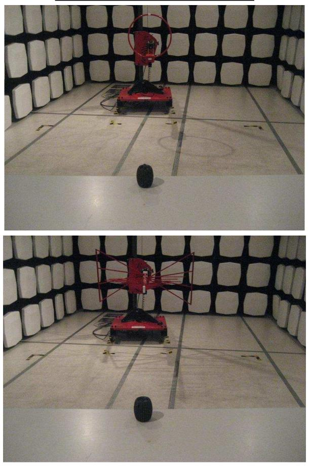
MEASUREMENT OF RADIATED EMISSION TEST SET UP
