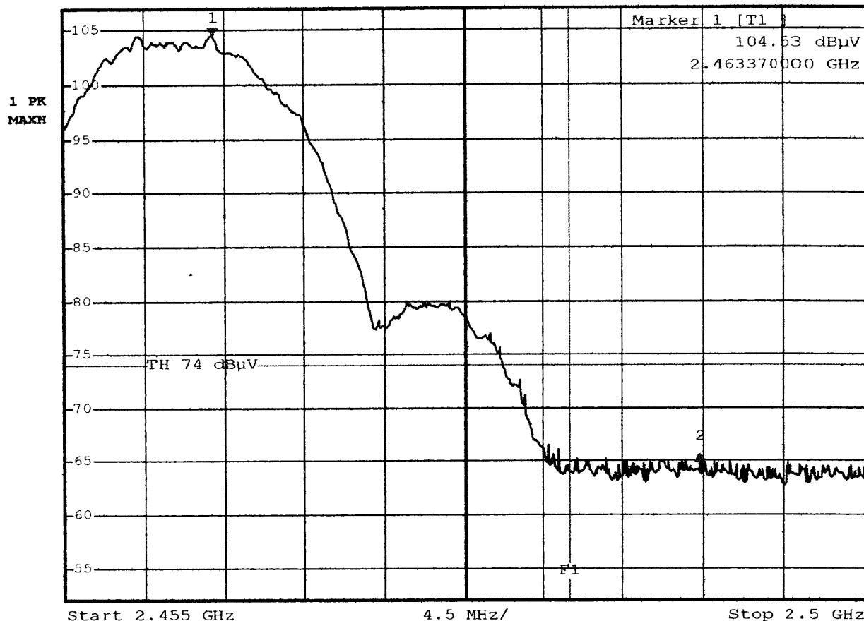
Comment A: Band-edge test at high channel
