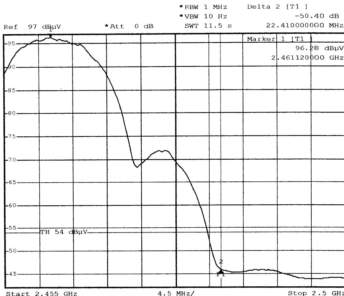
Comment A: Band-edge test at high channel F1=2483.5MHz
