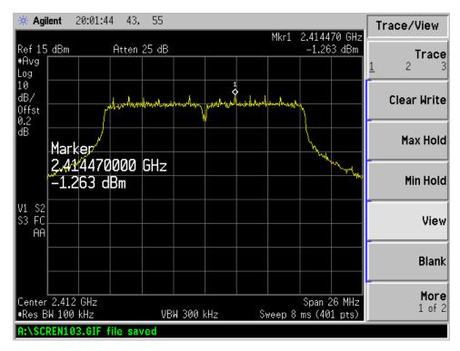
Result data graph shows middle channel power spectrum density is -1.382dBm at 100 KHz RBW
