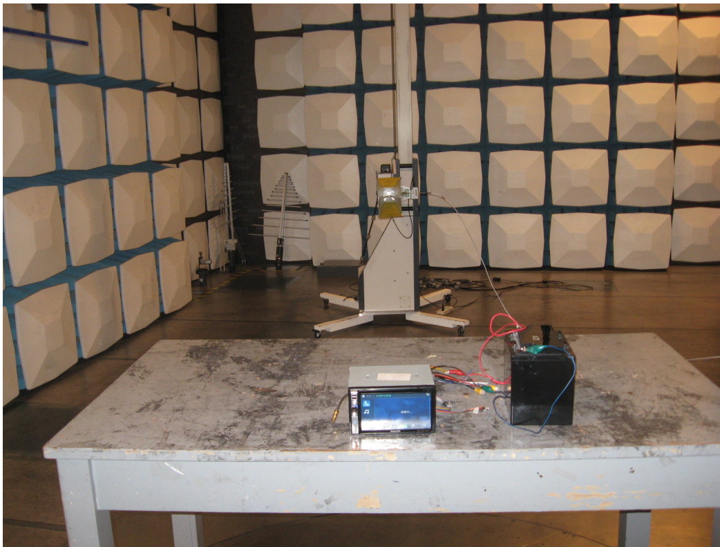
Photograph 2: Set-up for Radiation Measurement 1-18GHz
