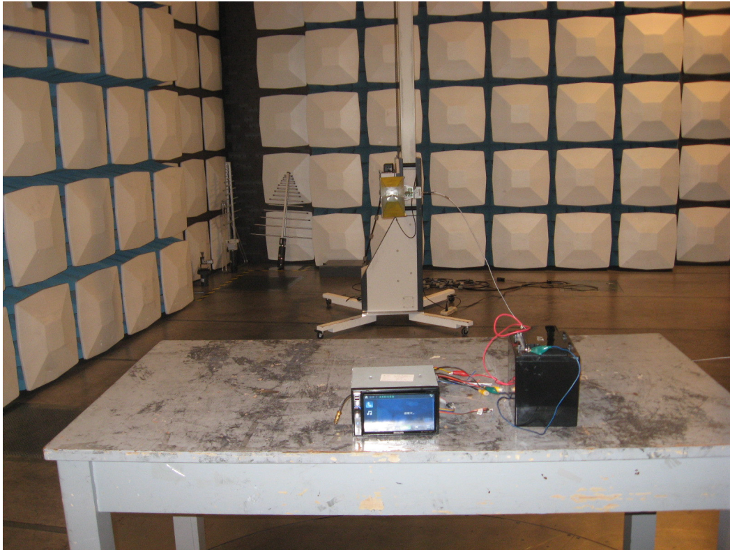
Photograph 2: Set-up for Radiation Measurement 1-18GHz
