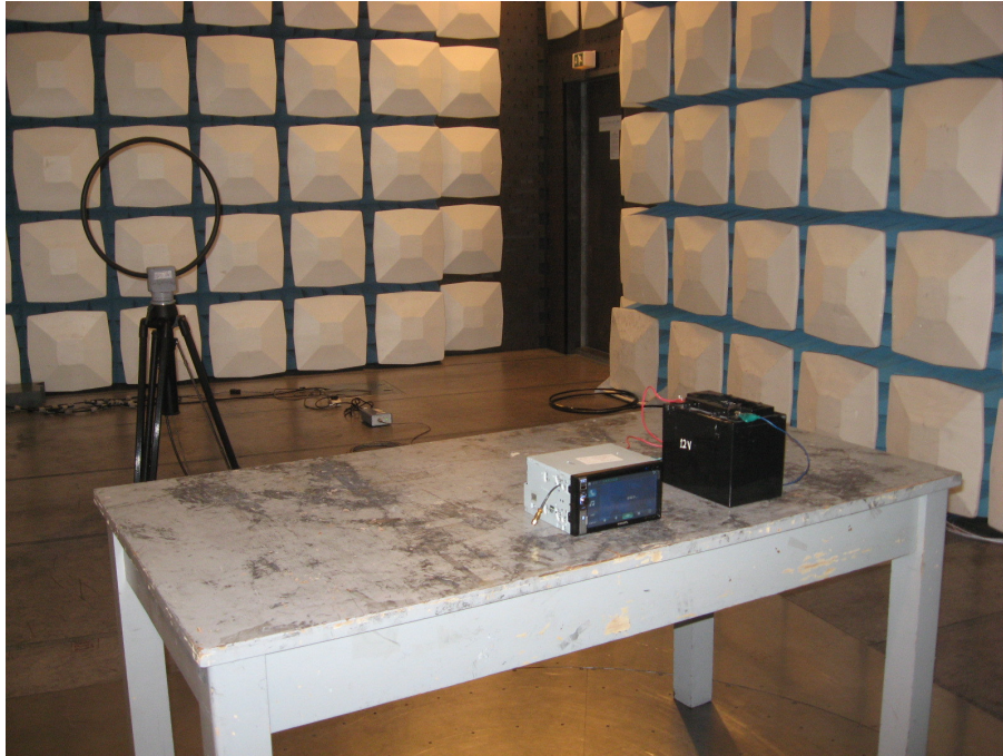
Photograph 1: Set-up for Radiation Measurement below 1GHz
