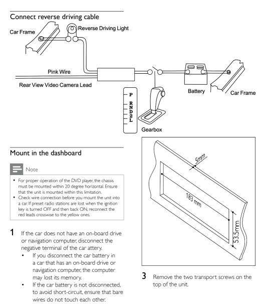
2 Ensure that car dashboard opening is within these measurements:
