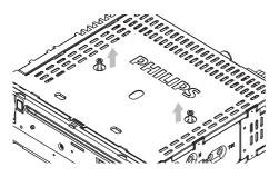
4 Remove the mounting sleeve with the removal keys.
