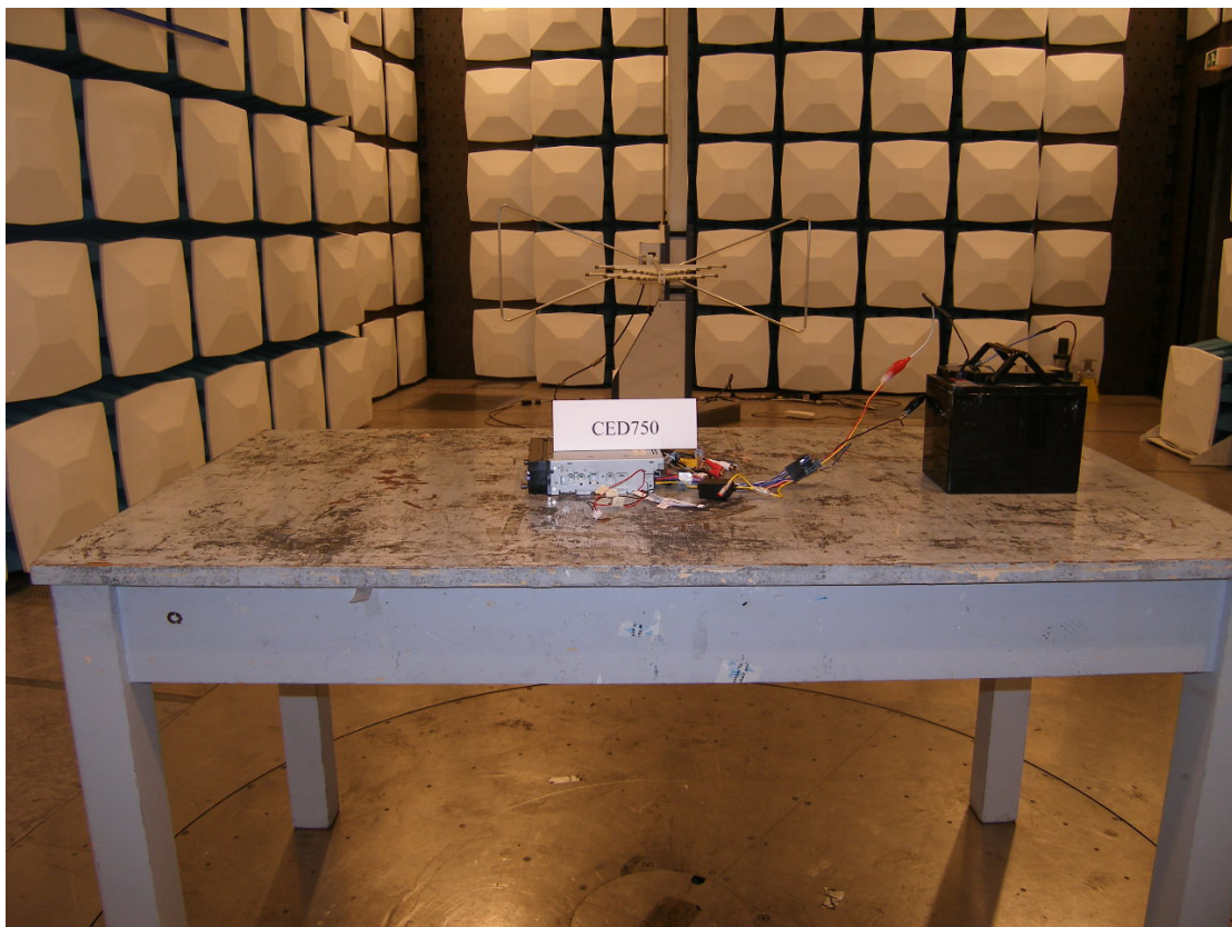
Photograph 1: Set-up for Radiation Measurement below 1GHz
