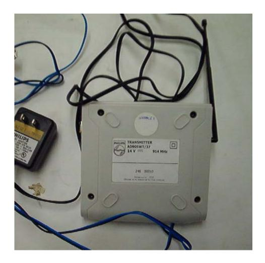
The model number label is located on the bottom of the Transmitter as pictured here.
