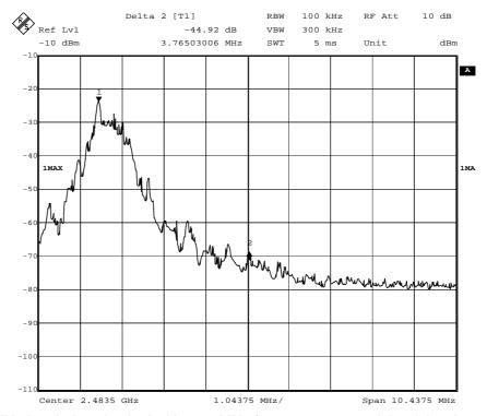
For 2483.5MHz bandedge checked with 2480MHz frequency operated, the delta shown at the plot are 45.04dB for peak detector mode and 44.92dB for Average detector mode.
