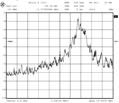
For 2400MHz bandedge checked with 2402MHz frequency operated, the delta shown at the plot are 39.79dB for peak detector mode and 39.74dB for Average detector mode.
