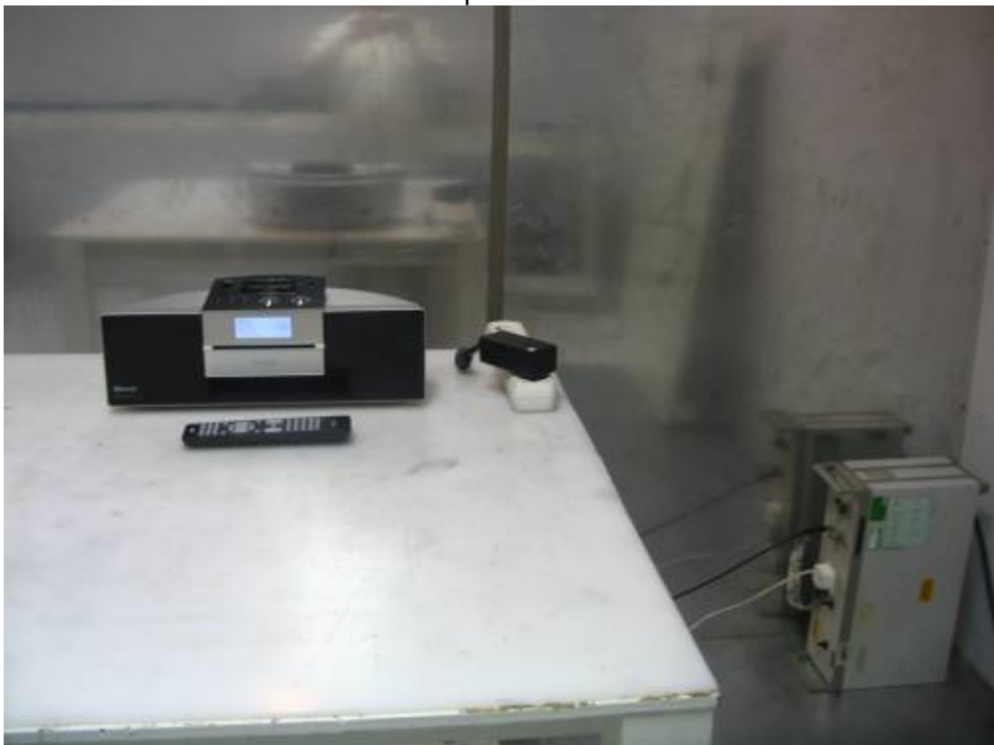
Conducted Emission Test Setup
