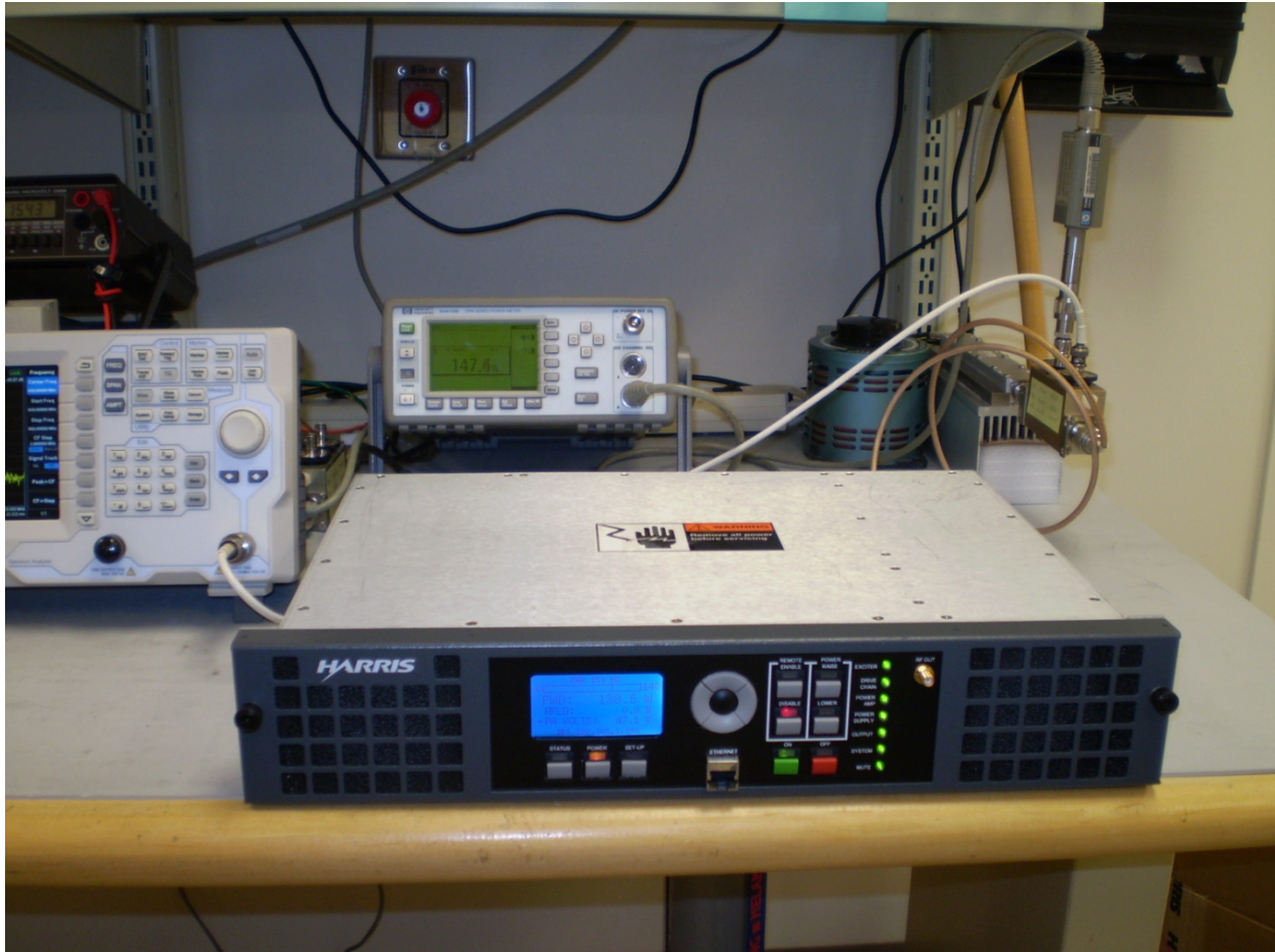
Figure 1, Load, Coupler, and Power sensor for conducted emissions and audio tests.
