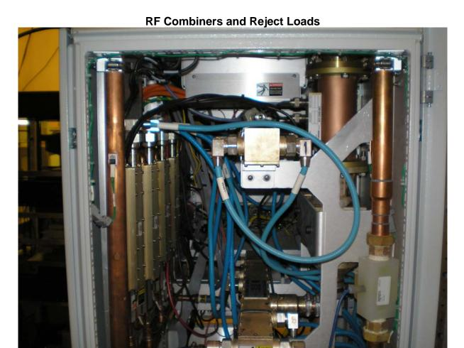
This photo of the rear upper area of the cabinet shows the two 3dB 4-way combining assemblies, above each other at the center, and the RF Load cooling plate on the left. Coolant lines from the cabinet connection points at the top of the cabinet can be seen at the left and the right. Coolant is distributed to all modules and to a cooling plate on which are mounted the reject loads.
