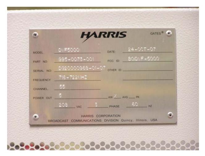
The plate is metal and is engraved as shown here. It is riveted to the DVF5000 and other models of the series in the location on rear door shown on the following page.
