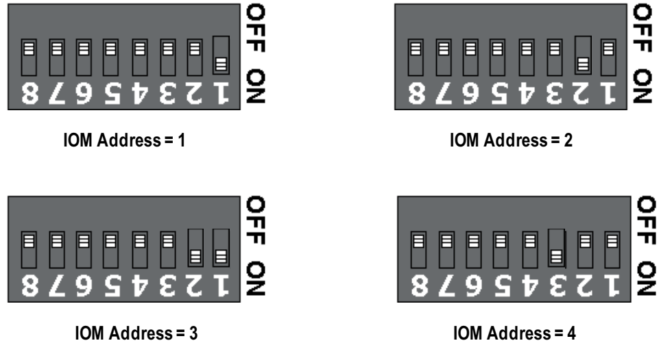
Fig. 32. IOM Address set up - S3 Settings
